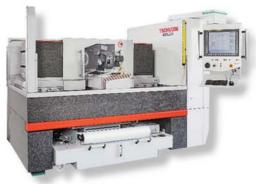
The centerless grinding machines of the TSCHUDIN 400 ecoLine / proLine series are optimally suited for machining medium-sized workpieces with diameters up to 150 mm
