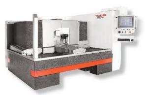
For large workpieces up to 250 mm in diameter and 500 mm in length, the TSCHUDIN 600 ecoLine / proLine is ideal
